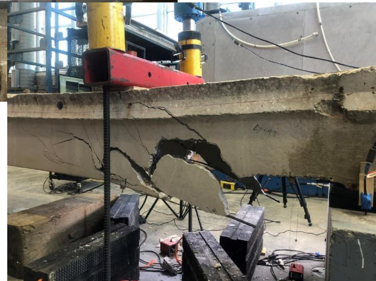
Severe Damage: 38.7 kips
