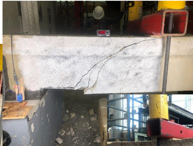
Intermediate Damage: 49.2 kips
