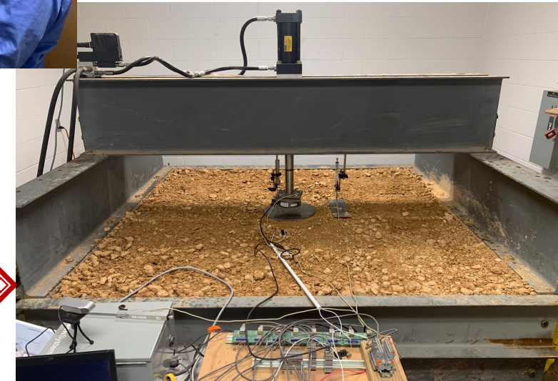
18-inch subgrade + 12-inch base
