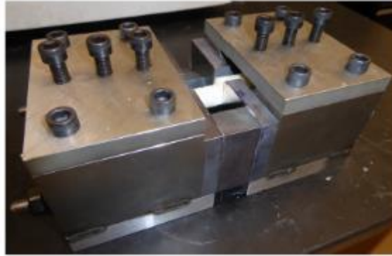
Transverse shear strength (ASTM D7617)
