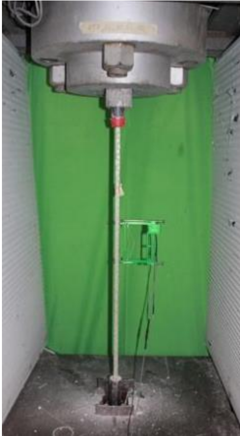
Tensile strength & E modulus (ASTM D7205)
