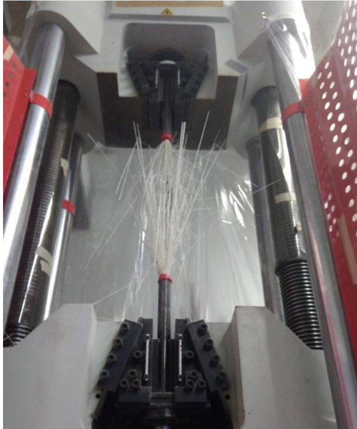
Tensile test post alkaline exposure without load
