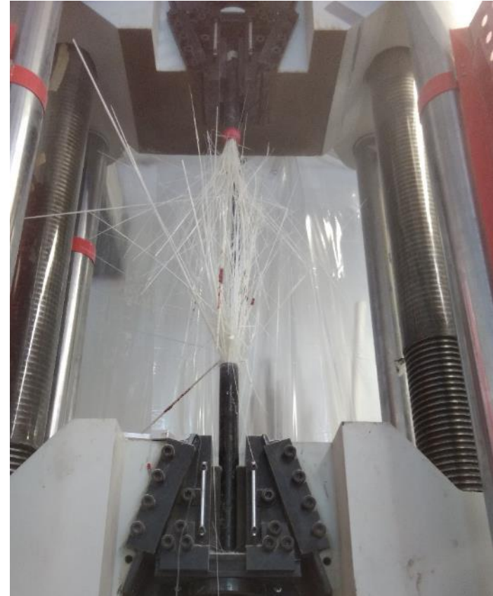
Tensile test post alkaline exposure with load
