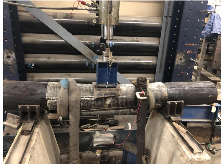
Shear Test on FRP Spliced Pile (typical failure mode)
