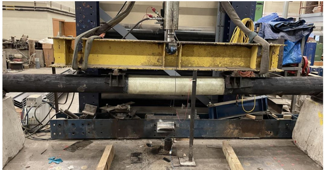
Improved FRP Splice Bending Test
