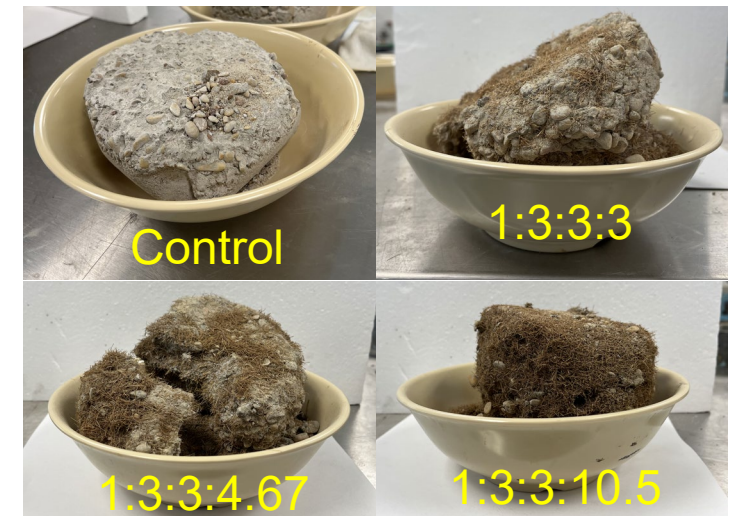
Concrete mixes after wetting and drying cycles
