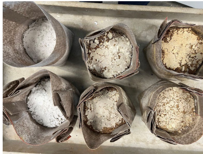
Concrete mixes during wetting and drying cycles
