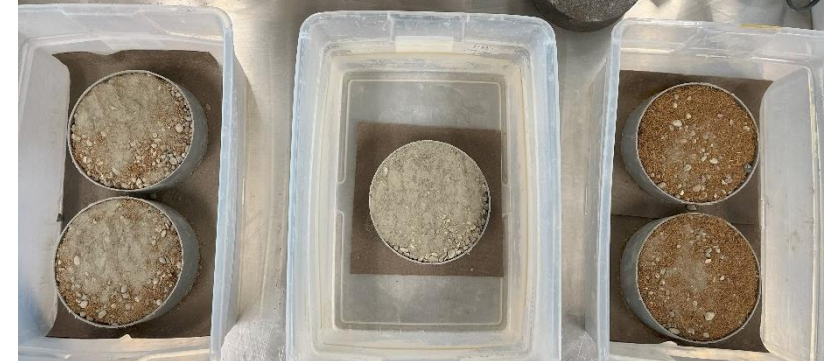
Dry concrete mixes samples in molds
