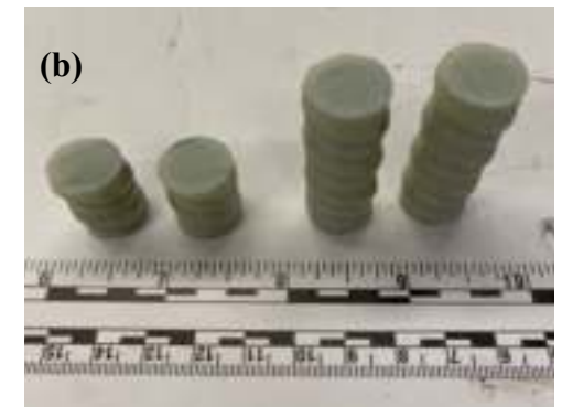
Tested GFRP bars: (a) G1 coupons; and (b) G2 coupons.
