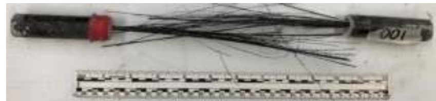
Fig. 1. Representative failure mode of tensile tests.
