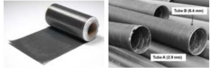
Fig.1. CFRP wrap 1 and filament wound FRP tubes 2 .
