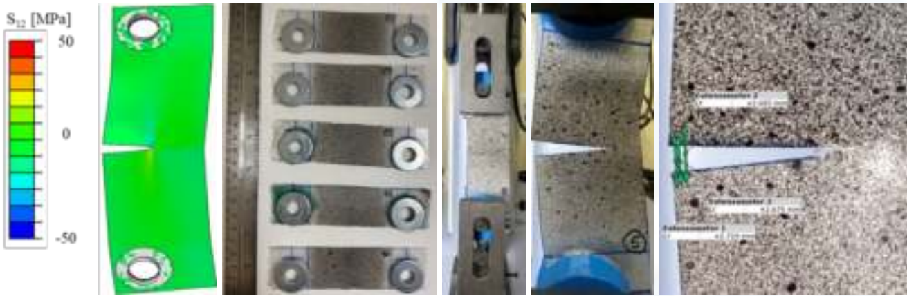
Experimental fracture test of a single layer Glass/epoxy composite based on ASTM standard [1]
