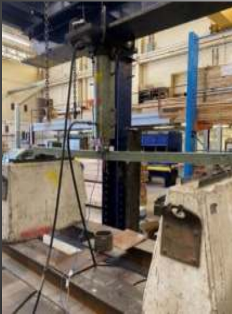
3-Point Bending of 3"×3"×0.5" specimen (84" span)
