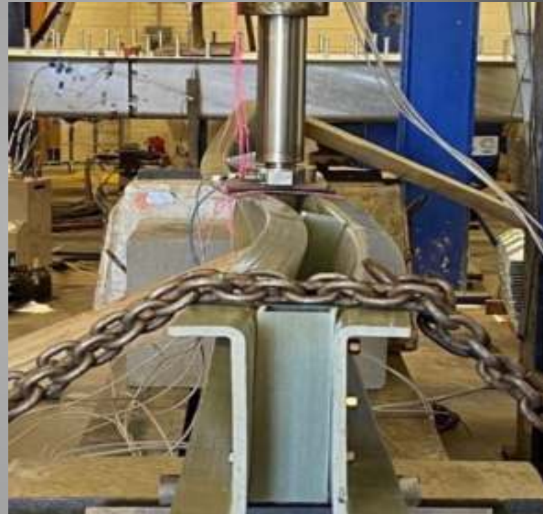
10"×2.75"×0.5" Back-to-back channels: lateral torsional effects under bending
