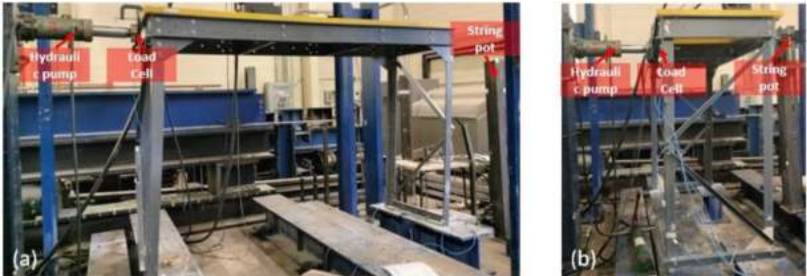
Test Setup for loading in long direction (a) and short direction (b).
