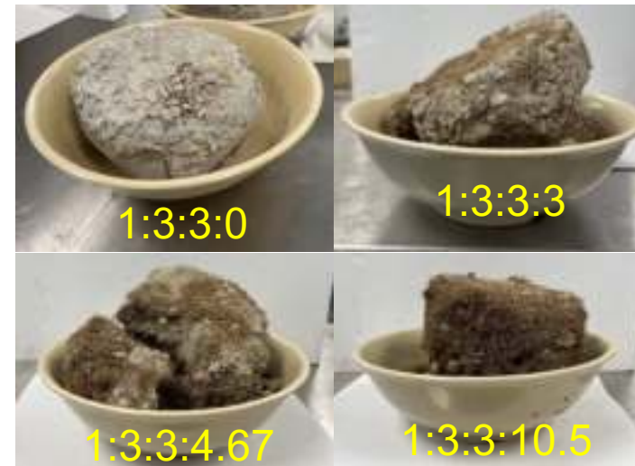
Concrete mixes after five wetting and drying cycles at 20 C
