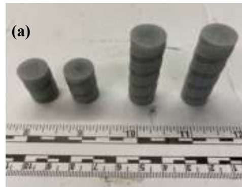
Tested GFRP bars: (a) G1 coupons; and (b) G2 coupons.
