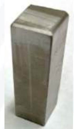
Square cross-section steel Impactor 17.8 x 17.8 mm [1]
