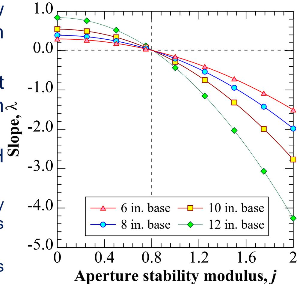
Slope vs Aperture stability modulus graph based on G-H equation
