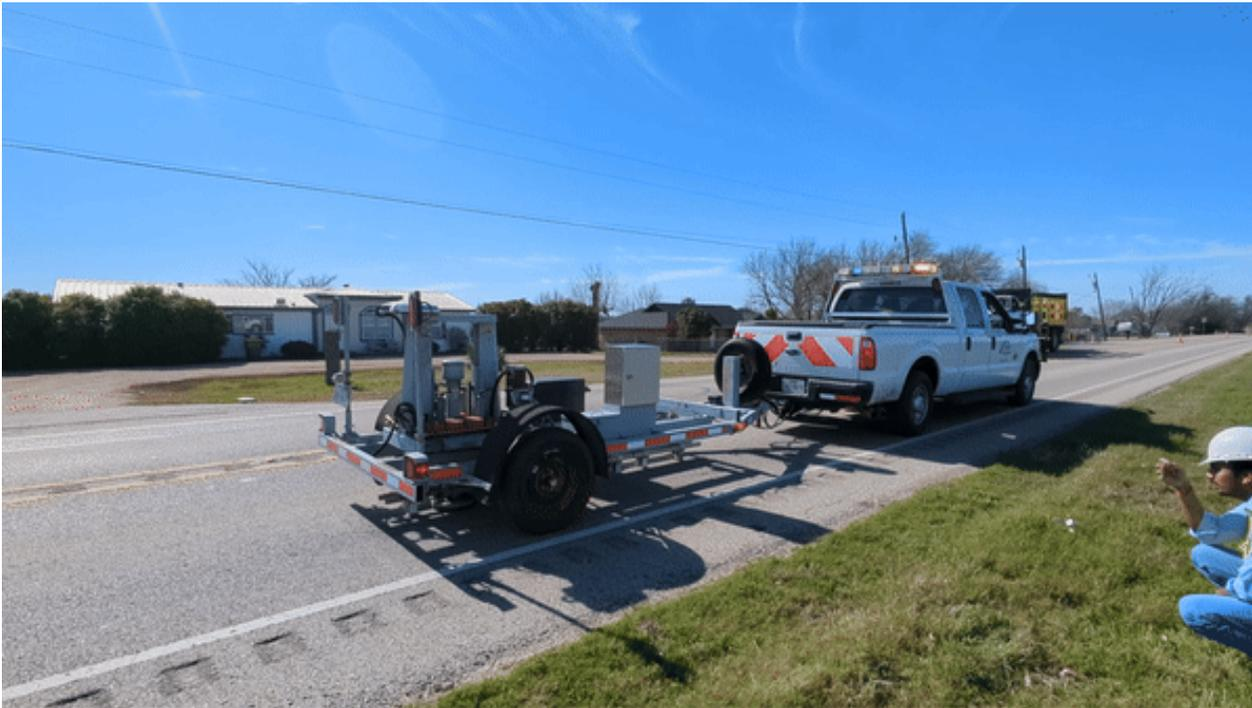
FWD Test on Field Test Sections
